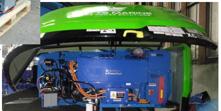
e-PowerPack installed into Genie S-45 XC
